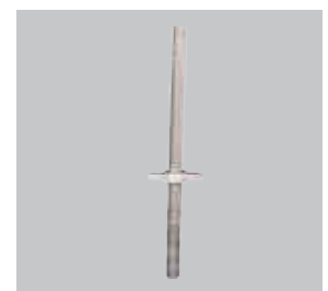
Universal Jack Connected on the top or bottom of the stander SWL= 40KN
